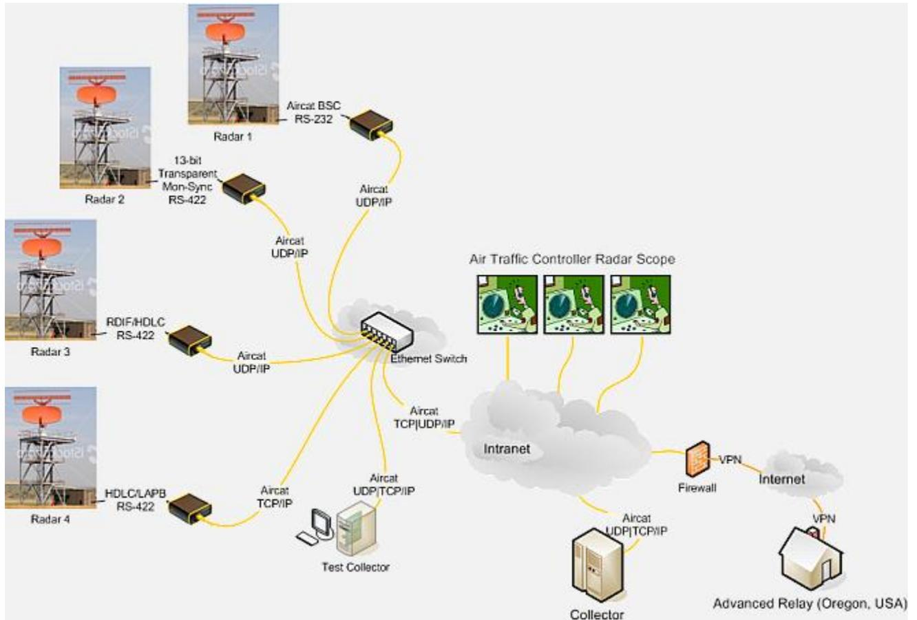
The radar system output is normally RS-422A. If an RS-232C narrowband microwave radio modem is used to connect to the local airport, an RS-422-to-RS-232 converter is needed. If an intranet connection can be established at the radar site, Advanced Relay's [PXSe](#) can directly
