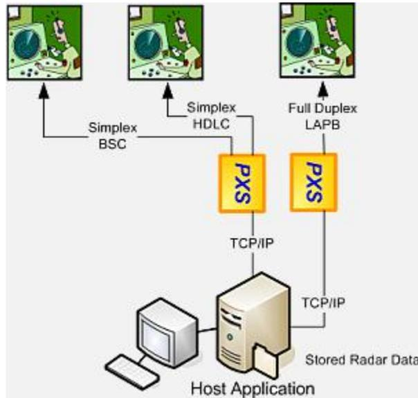
[Air Navigation and Weather Services \(ANWS\) Taiwan](#) uses the PXSe as a gateway from transparent bit stream (13-bit SYNC character) to TCP/IP. We developed a special Monosynchronous driver to handle the special bit-synchronous mode.
