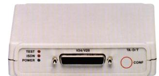
If no bonding of ISDN B-channels is used, the likely speed will be 64 kbps, but it is possible that the speed from the Host to the ISDN Terminal Adaptor is slower. If the speed to the Host is higher than 19.2 kbps, it is less likely that RS-232 (V.24) is used.
